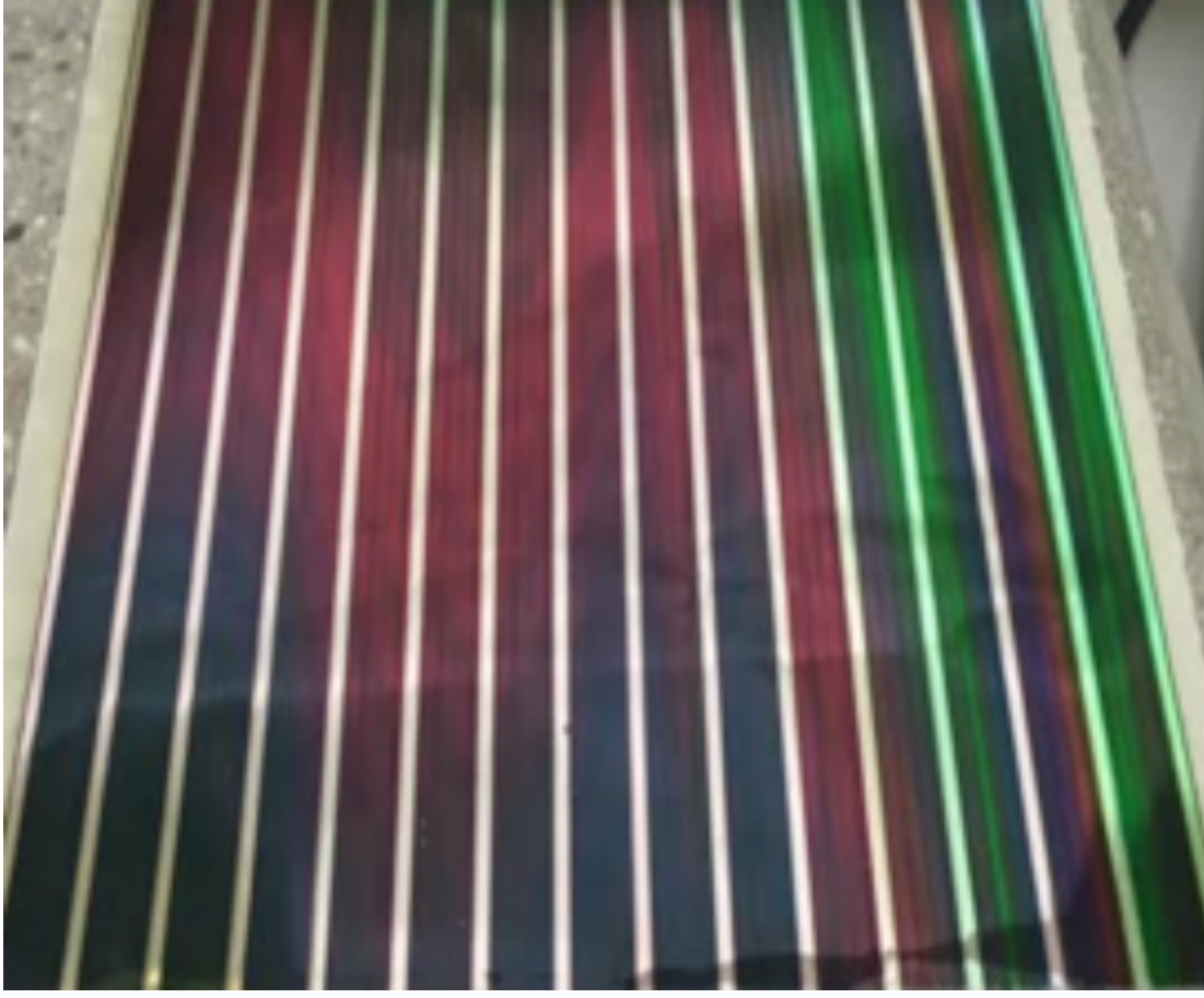
12" x 12" Card Segmented from the Mother Capacitor
